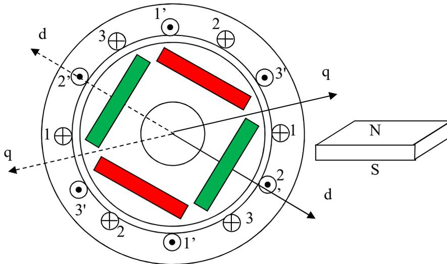
Figure 8-28: Example of IPM (Interior Permanent Magnet) synchronous machine, 4 poles (green magnets have North outward while the South towards the rotor; red ones vice versa)
