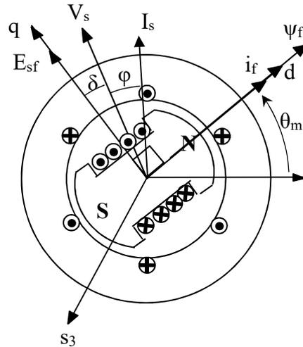
Figure 8-22: machine with salient poles (anisotropic machine)
