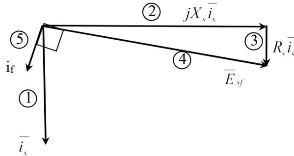
Figure 8-9. Phasor diagram of a synchronous machine in short-circuit condition
