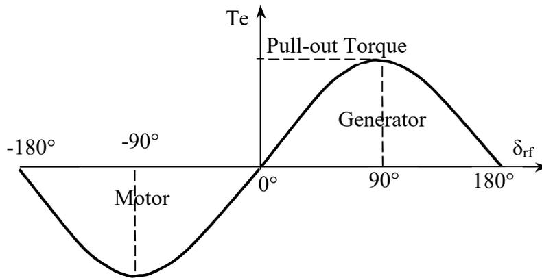
Figure 8-5: Electromagnetic Torque
