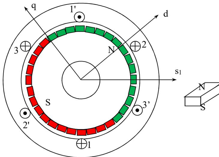
Figure 8-27: Example of a SMPM (Surface Mounted Permanent Magnet) synchronous machine, 2 poles (green magnets have North outward while the South towards the rotor; red ones vice versa)
