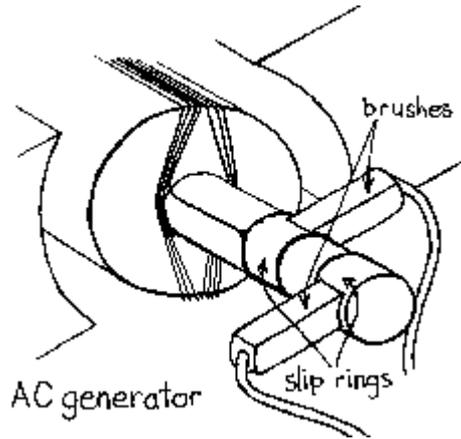
Figure 8-3: slip rings (<http://www.lselectric.com/>)
