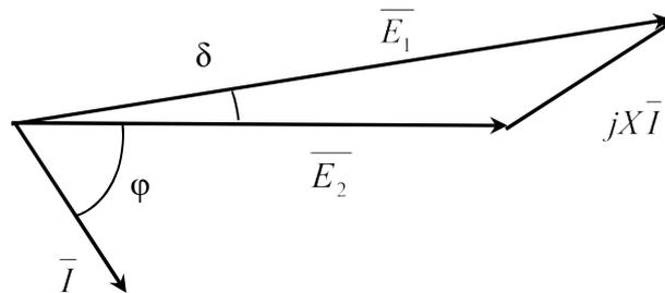
Figure 8-13. Phasor diagram of the simple equivalent circuit (no voltage drop on the resistance)
