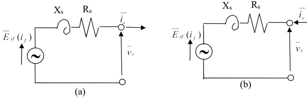
Figure 8-7: Equivalent circuit of an isotropic machine ((a) generator, (b) motor)
