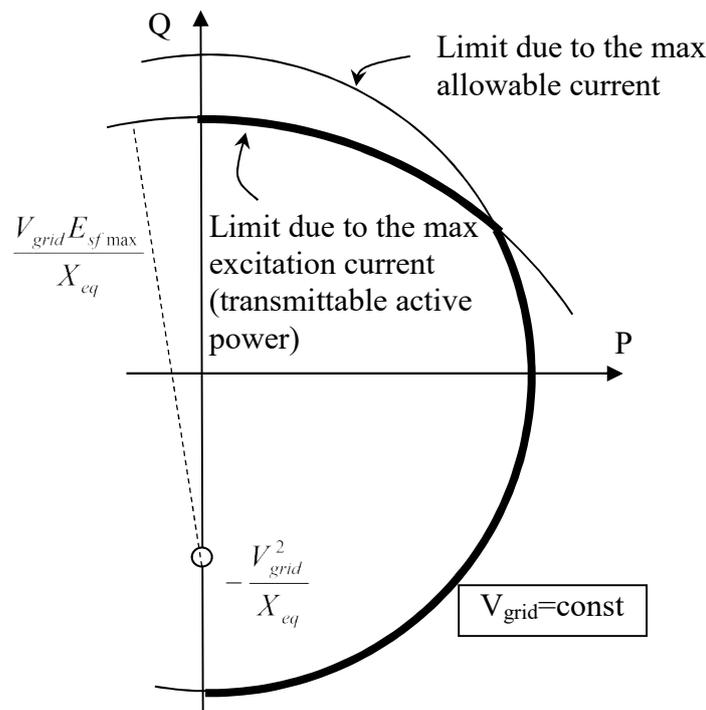
Figure 8-21. Limits due to the maximum currents
