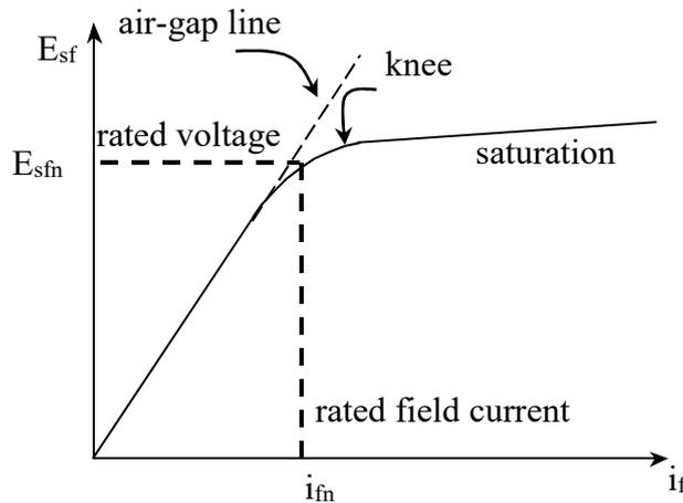
Figure 8-8: Open-circuit (no-load) characteristic of a synchronous machine
