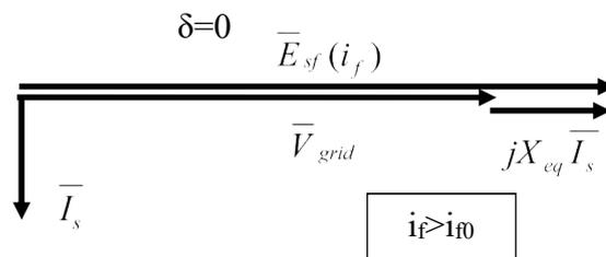
Figure 8-16. Phasor diagram in over-excitation condition
