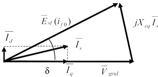
Figure 8-18. Phasor diagram with positive input mechanical power
