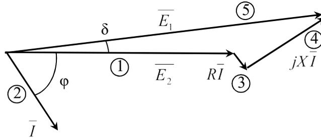
Figure 8-12. Phasor diagram of the simple equivalent circuit (the current is lagging the voltage  $E_2$ )
