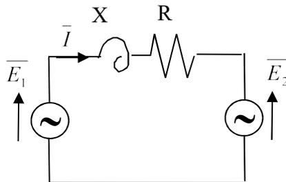
Figure 8-11. Simple equivalent circuit
