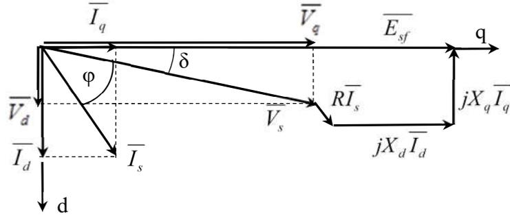
Figure 8-24. Phasor diagram for a salient poles machine (the axes are rotated by 90°)
