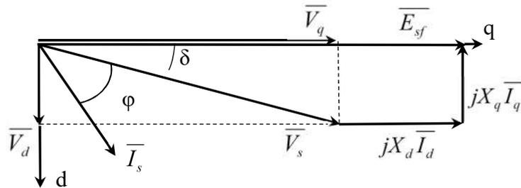
Figure 8-25. Phasor diagram for a salient poles machine (neglecting  $R_s$  effect)
