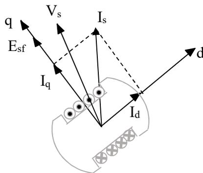
Figure 8-23: synchronous machine with salient poles (anisotropic machine), rotor only
