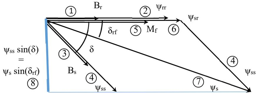
Figure 8-4. Phasor diagram of a synchronous machine
