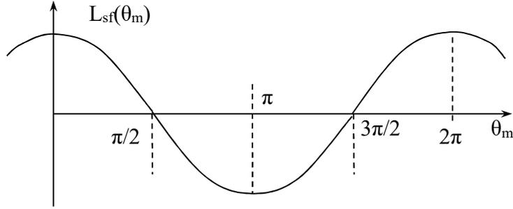
Figure 8-6: Waveform of the mutual inductance between the excitation and stator windings
