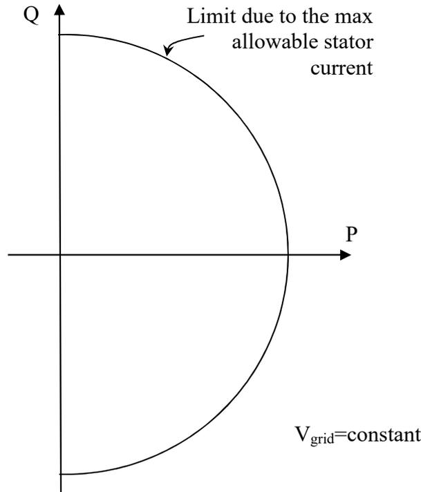
Figure 8-20. Limits due to the maximum stator current
