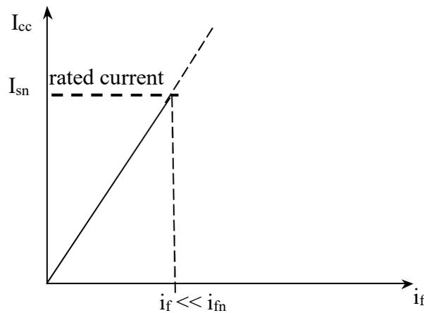
Figure 8-10. Short-circuit characteristic
