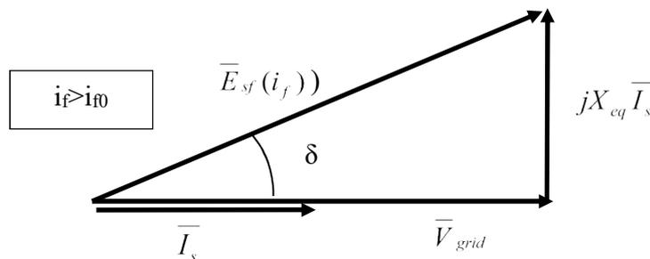
Figure 8-19. Phasor diagram with positive input mechanical power and no reactive power
