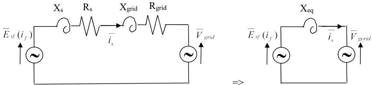
Figure 8-14. Equivalent circuit of a synchronous machine connected to the grid
