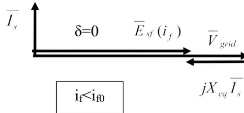
Figure 8-17. Phasor diagram in under-excitation condition
