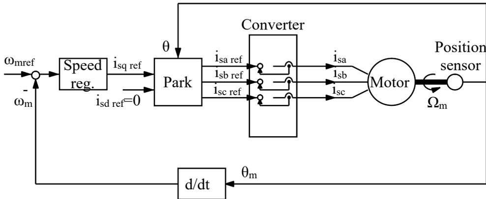
Figure 6-13: Speed control loop (current controlled power converter)
