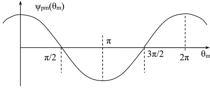
Figure 6-7: Waveform of the flux linked with the stator windings due to the PM
