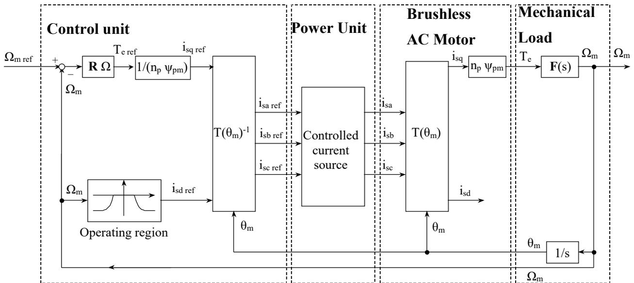
Figure 6-14: Full control scheme (current controller power converter)
