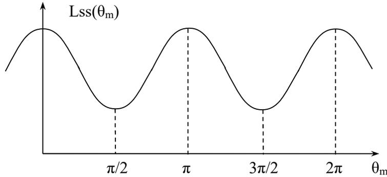
Figure 6-5: Self inductance behaviour of the first winding
