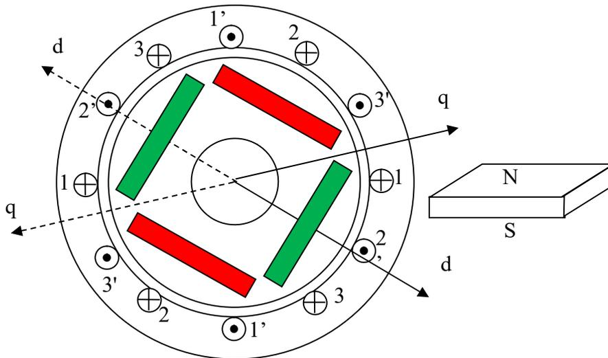
Figure 6-4: Example of IPM synchronous machine, 4 poles (green magnets have North outward while the South towards the rotor; red ones vice versa)
