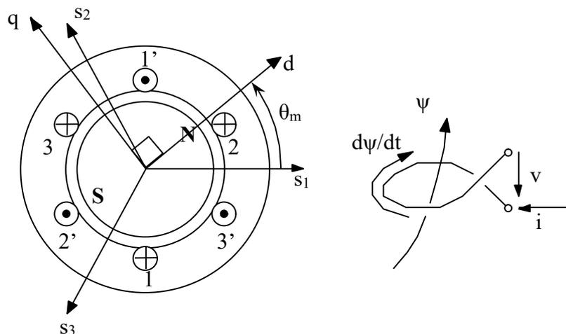
Figure 6-2: Schematic diagram of the brushless motor
