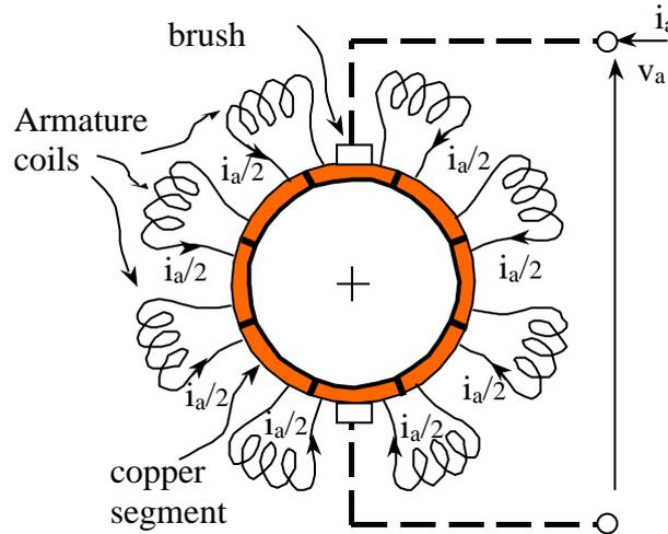
Figure 1-5. Commutator with 8 copper segments and 2 brushes
