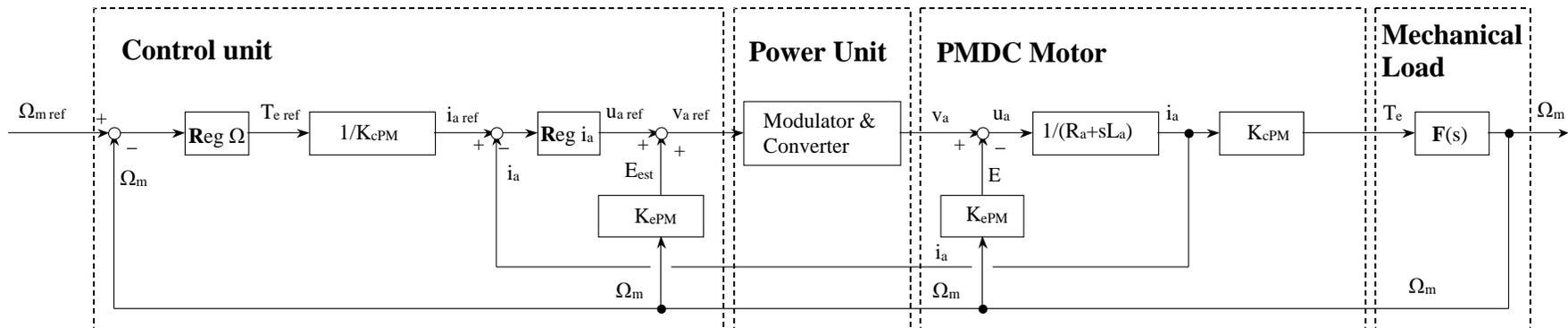
Figure 1-23. Speed control scheme of a PM DC machine (controlled voltage source)
