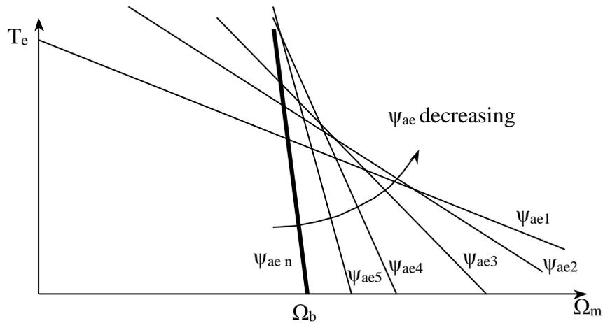
Figure 1-16. Mechanical characteristics (torque vs speed) as a reducing of the flux  $\psi_{ae}$  (weakening operation of the machine)
