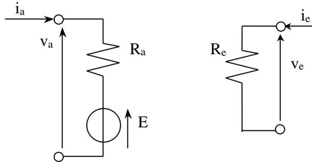
Figure 1-13. Steady state equivalent circuit of a DC machine
