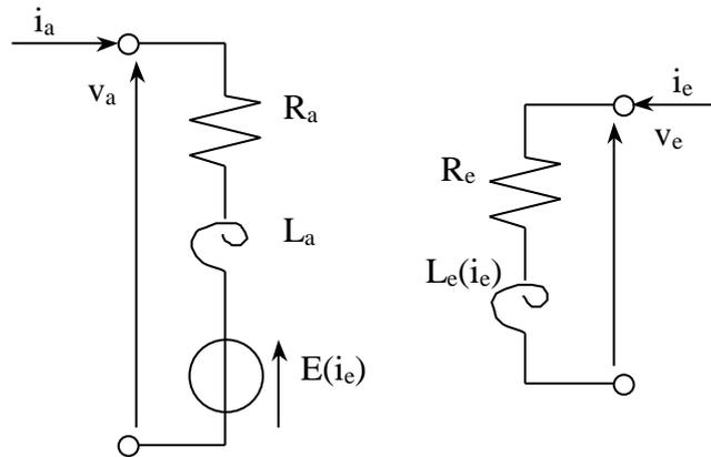
Figure 1-12. Dynamic equivalent circuit of a separately excited DC machine
