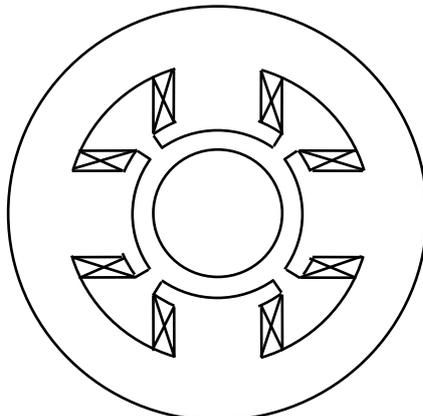
Figure 1-4. Four poles, separately excited, DC machine cross-section
