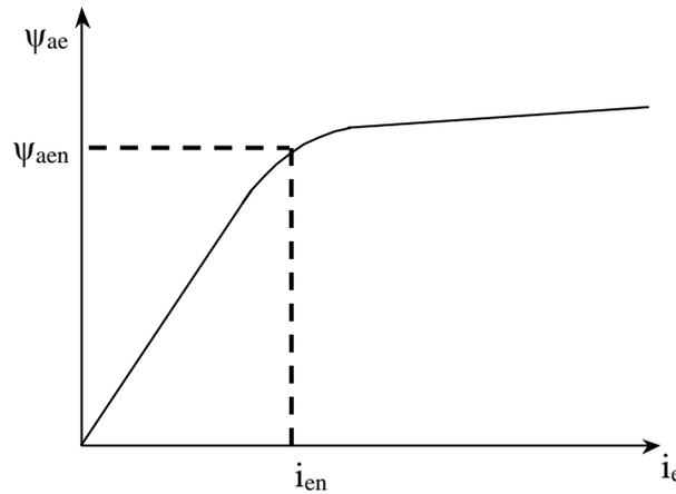
Figure 1-15. Non-linear relationship  $\psi_{ae} = g(i_e)$ ;  $i_{en}$  = rated value of the excitation current,  $\psi_{aen}$  = rated value of the flux  $\psi_{ae}$
