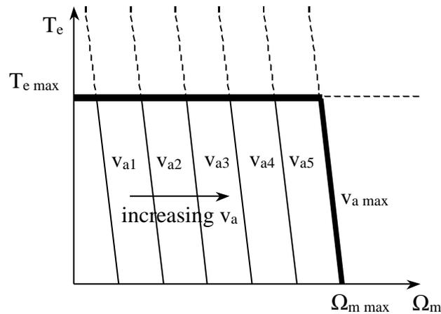
Figure 1-14. Torque/speed characteristics as a function of the armature voltage, and operating regions
