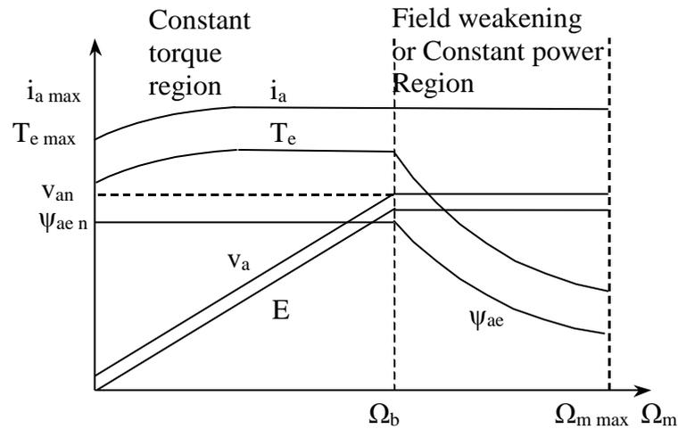
Figure 1-18. Operating regions with a cooling system whose efficiency depends on the mechanical speed
