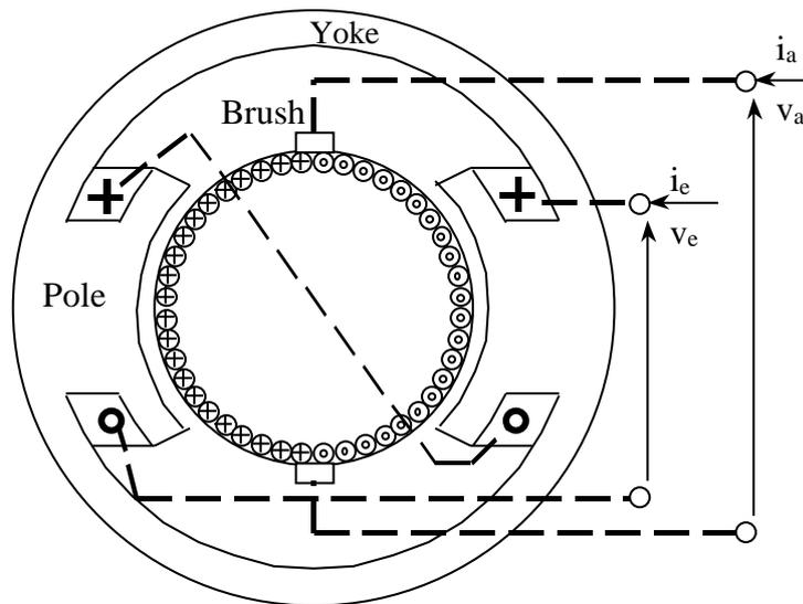
Figure 1-2. Two poles, separately excited, DC machine cross-section
