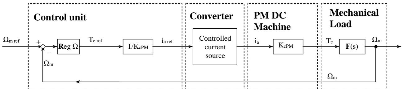
Figure 1-21. Speed control scheme of a PM DC machine (controlled current source)
