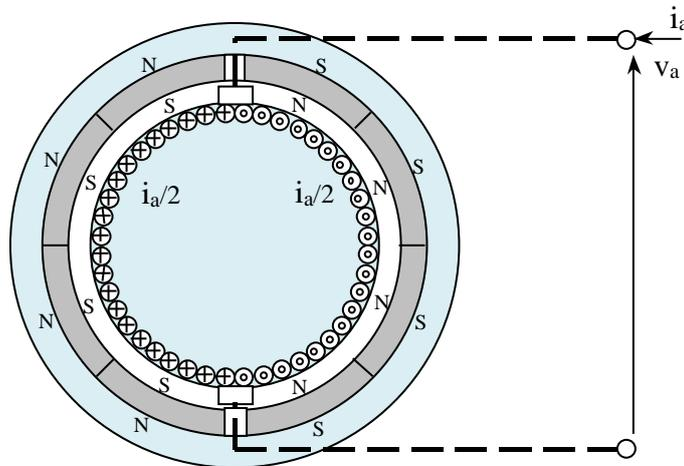
Figure 1-3. Two poles PM DC machine cross-section
