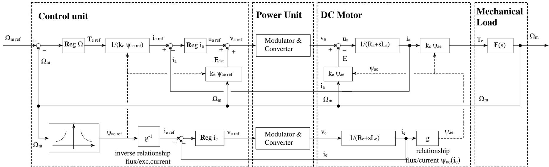
Figure 1-22. Speed control scheme of a separately excited DC machine (controlled voltage sources)
