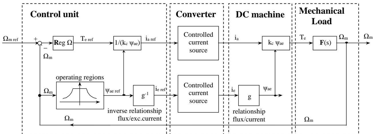
Figure 1-20. Speed control scheme of a separately excited DC machine (controlled current sources)
