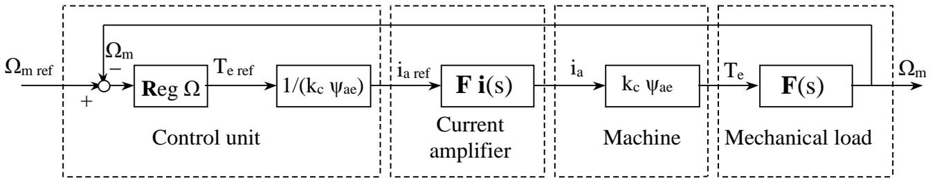
Figure 1-26. Scheme for the speed regulator design
