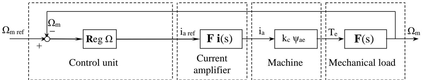
Figure 1-27. Scheme of the mechanical speed regulator without any adaptive term
