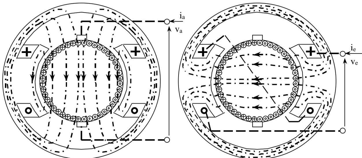
Figure 1-11. Development of magnetic field lines inside the machine
