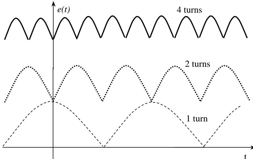
Figure 1-10. electromotive force waveform with two brushes and a commutator with: two semi-rings (1 turn), 4 segments (2 turns), 8 segments (4 turns)
